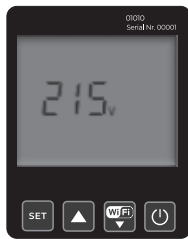
Undervoltage/ Overvoltage Setting
